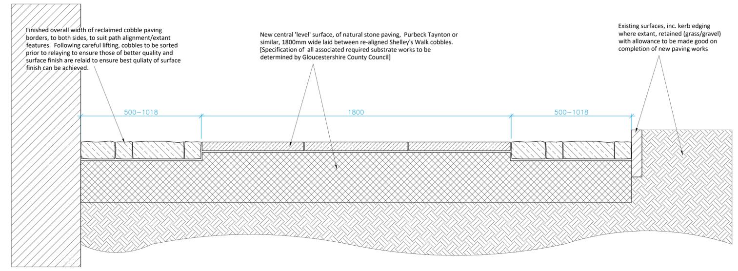
Indicative section (looking east) through re-laid section of path (~1:10)
